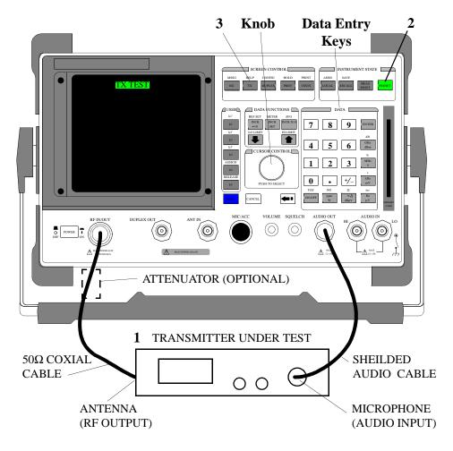
1. Connect the Transmitter as shown.
