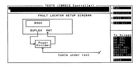
13. Follow the displayed instructions to connect and remove the 50  $\Omega$ Termination at the Power Divider cable test port. Remember to select **Continue** after each step.
