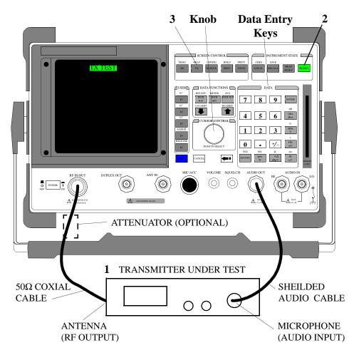
1. Connect the Transmitter as shown.
