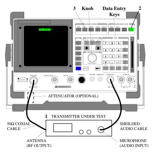
1. Connect the Transmitter as shown.
