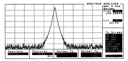
Relative frequency and amplitude measurements such as filter bandwidth, duplexer rejection/insertion loss, or harmonic level can be performed using the "Delta" marker function.
